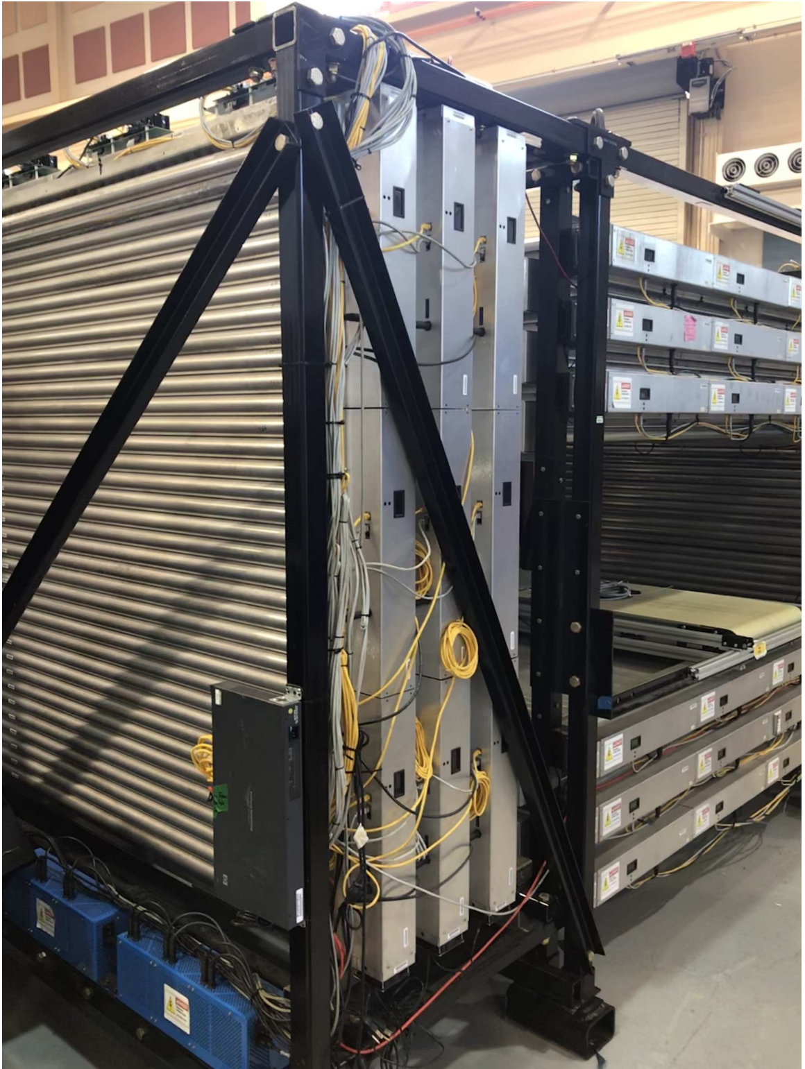
Figure 9.2: The new drift tube detector at Los Alamos National Laboratory.
